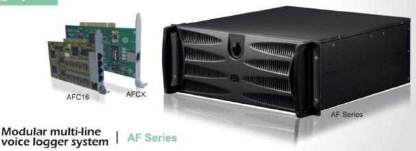
AF series is high-end voice logger based on industrial-grade computer. Each AF voice logger starts from 16 channels and is expandable up to 150 channels. It works with 5 voice cards includes
